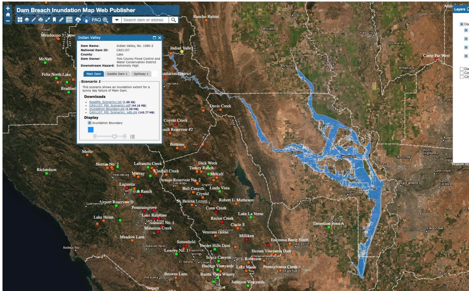
Dam inundation zone for the Indian Valley Reservoir (High-Risk).
